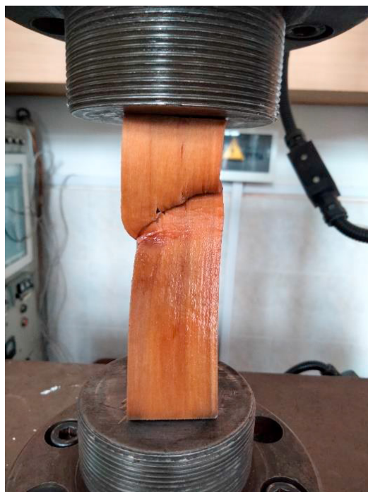
Fig 1. Destruction of a birch wood prism under the action of lactic acid (40%) with a soaking time of 28 days
