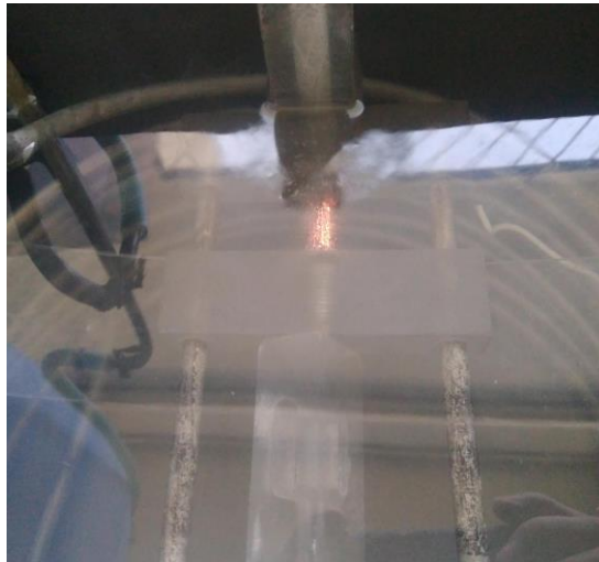
Fig. 1. Synthesis of oxide ceramic coating in spark discharge plasma on a titanium alloy sample
