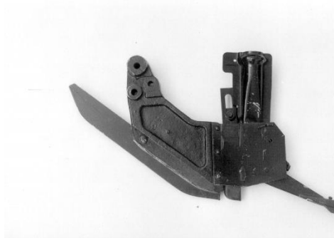
Figure 2. A runner coulter of grain seeder
