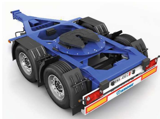
Fig. 2. 2-axle trolley “Dolly” with fixed axles (trolley trailer) from “KRONE” company [10].
