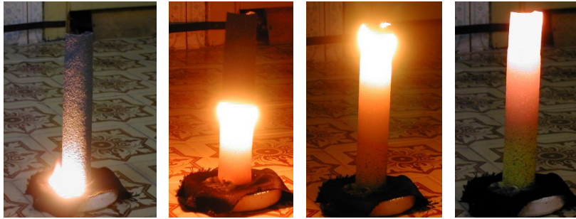
Fig.4. Obtaining PPM on the basis of Ti + C with the help of SHS - process
