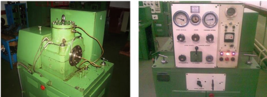
Fig. 2. Installation of VNIPP-542 to test the wear resistance of bearings.
