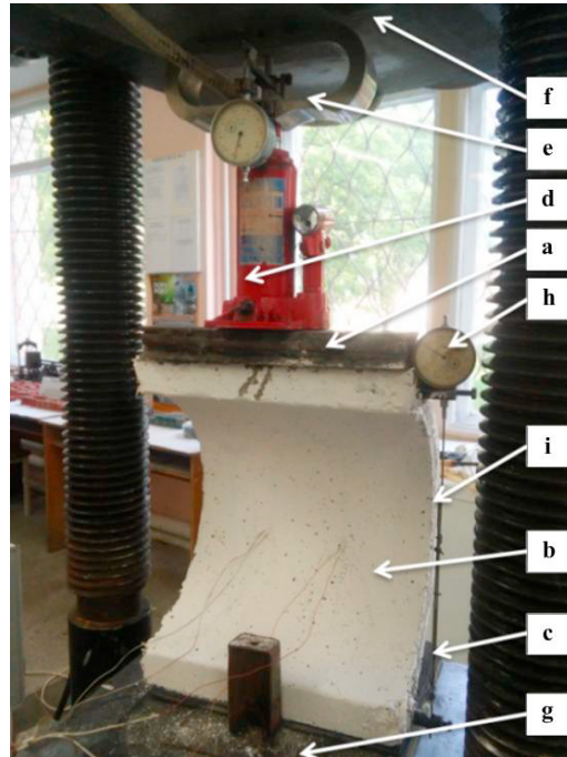
Fig. 2. General view of the drainage gutter test. (a) steel loading beam; (b) tested drainage gutter; (c) fixed support; (d) hydraulic jack; (e) reference dynamometer; (f) upper plate of the PSU-125 press; (g) lower plate of the PSU-125 press; (h) displacement sensor and (i) displacement rod
