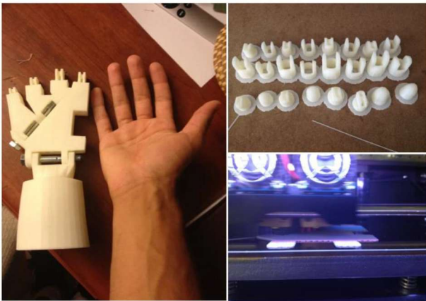
Fig. 12. Stages of manufacturing a mechanized humanoid robot arm: size comparison with a human arm, set of printed parts and 3D printing process
