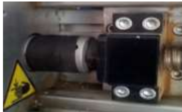
Fig. 16. Adjusted coupling connecting the stepper motor to the Y-axis lead screw
