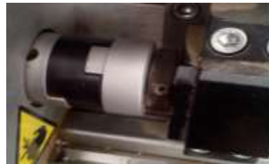
Fig. 15. Worn coupling connecting the stepper motor to the Y-axis lead screw
