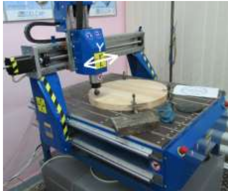
Fig. 1. Experimental CNC milling machine with 3-axis numerical control system
