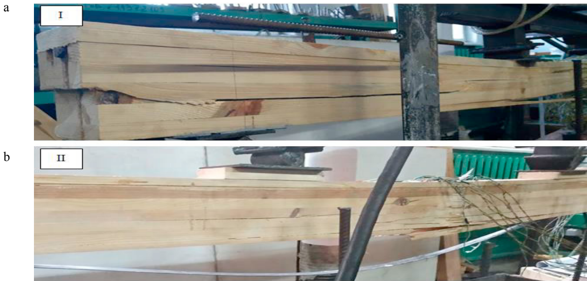
Fig. 8. Nature of failure of reinforced beams: (a) GRB-12 (Prst) beam with pre-stressed composite reinforcement; (b) GRB-12 beam without pre-stressed reinforcement.
