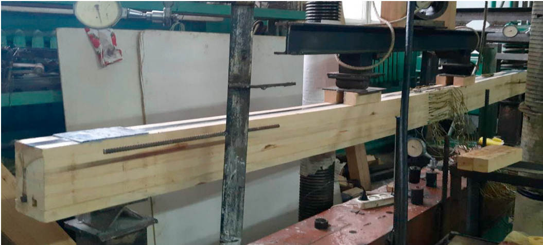
Fig. 3. Wooden beam GRB-12 (Prst) under loading during the pre-stressing process of the composite reinforcement.
